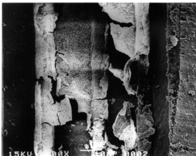
Figure 3. SEM image of ureteral stent recovered from a patient. The stent was opened longitudinally to show the extent of encrustation which was almost sufficient to block the flow of urine.
